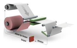
Regulation in torque with dancing roller for splicer systems
