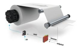
Regulation in torque with load cells
