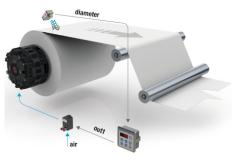
Regulation in torque with diametral sensor (open-loop)
