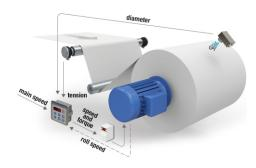
Regulation in torque/speed with load cells or dancing roller for motorized unwinders/rewinders
