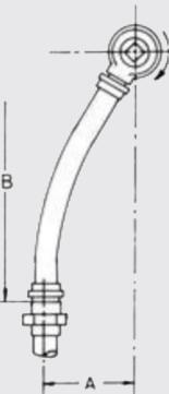
The correct way to install the hose on a rotary union
