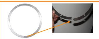
HSS cutting ring can be opened and removed from the shaft.
