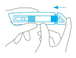
Finally, push the plastic insert back into the handle until you hear it click into place
