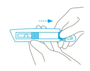
Press the blade-change button and **pull out** the plastic insert.
