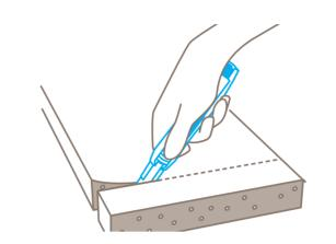
**Depending on your cutting job** leave your thumb at first on the slider to fix the blade.
