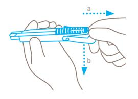
Pull the blade change button to the back as marked by the arrow (a), flip the end of the handle downwards (b) and **move the blade out of the handle** by using the slider.
