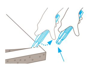
Always **remove your thumb** from the slider at the end of your cutting job to ensure automatic blade retraction. **Always cut past your body.**
