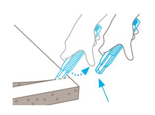
Following cutting, the blade immediately retracts into the handle. CAUTION: **Don't block** the slider with your hand.
