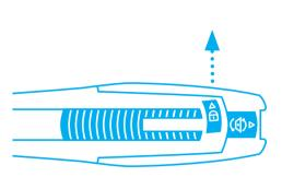
To lock the slider shut, **push the safety device** upwards as marked by the arrow.
