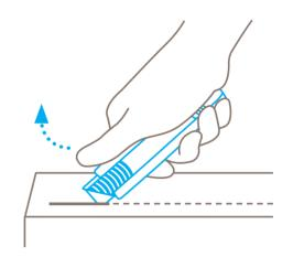
Remove your **thumb from the slider** to ensure automatic blade retraction.
