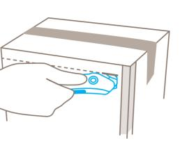
Use the nose of the cutter to **pierce** the cutting material. Do not lever against staples, nor force the nose into edge protectors!
