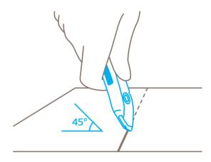
Hold the cutter at a **slight angle** when cutting through cardboard boxes.
