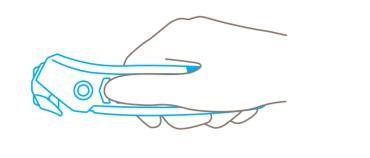
For the best possible grip, place your thumb on the **three ribs**. The soft-grip further limits the possibility of slipping.
