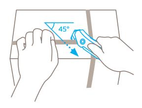
For best results, cut plastic strapping band diagonally (at a 45° angle).
